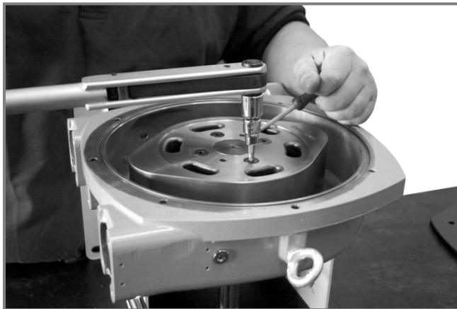
Figure 10 Installing the rotor
